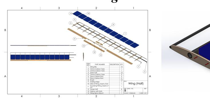
Most design iterations occurred around the mounting configuration of the solar cells within the wing. The prototype features the cells connected with pre-bent wires resting on the wing ribs.
